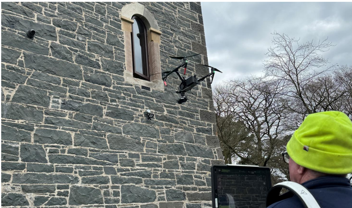
Helen's Tower, Drone surface survey in action © Roger Perrott
