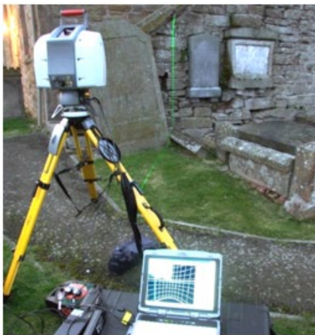
Figure 12: Laser Scanning in operation. Photo: Historic Scotland
