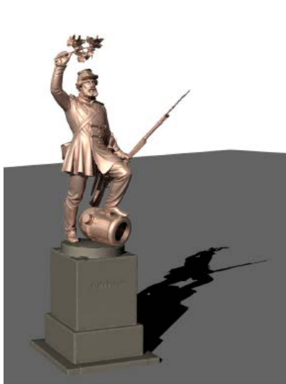
Laser Aided Modelling (LAM®) to feed into BIM3D model. Detailed Forms: Generated with a VR Mesh. Illustration: Ramboll
