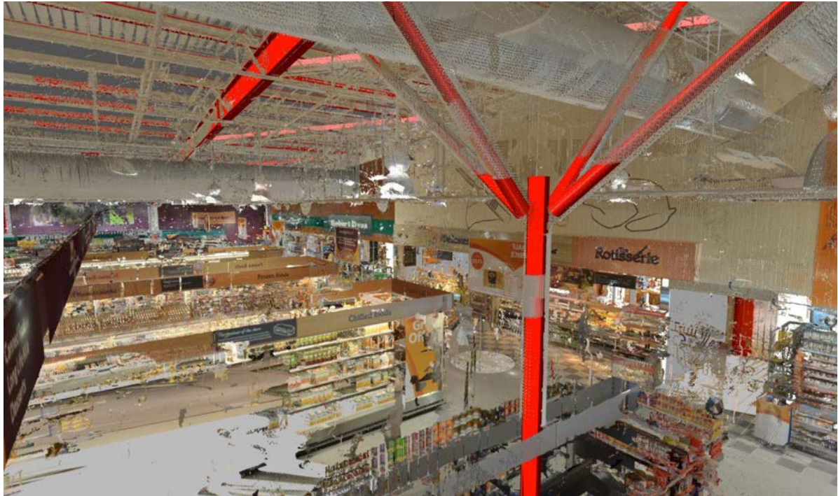
Laser Aided Modelling (LAM®) 3D Structural Arrangements: Extracting Steel Sections Illustration: Ramboll
