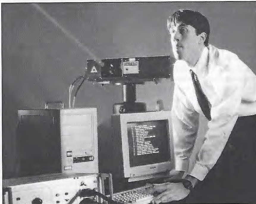
BRE 3D-laser survey system
